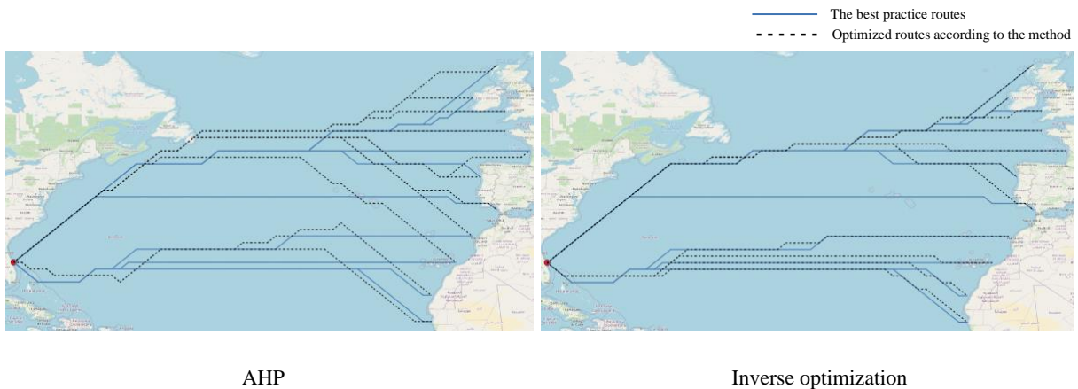
Figure 11. Comparison of the best practice routes (blue line) with the optimized route (dotted lines) through AHP and inverse optimization methods.
